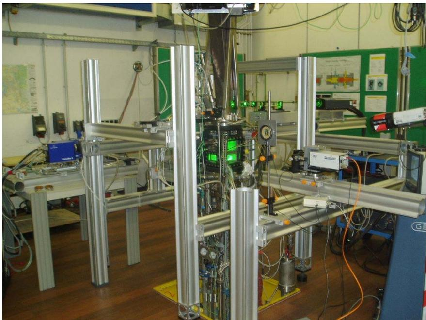
Single sector combustion test facility illuminated by a PIV laser light sheet. The PIV camera system is visible to the right of the combustion chamber.
