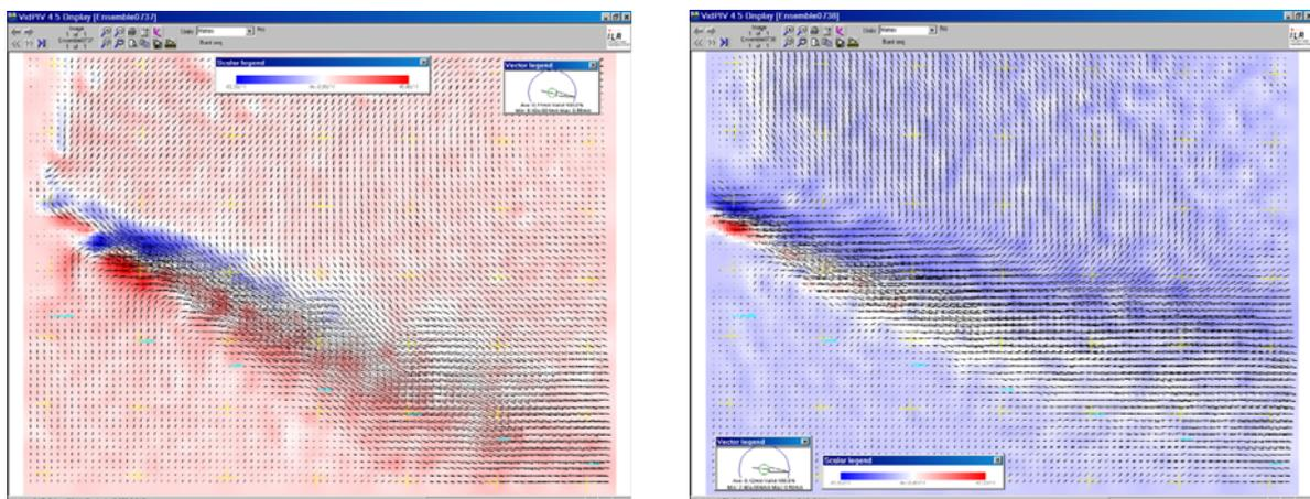
Evaluated PIV images of a steel casting process without bubbles (left) and with bubbles (right). The mean mean shaer strain in the flow is shown above which has been derived from the velocity field.
