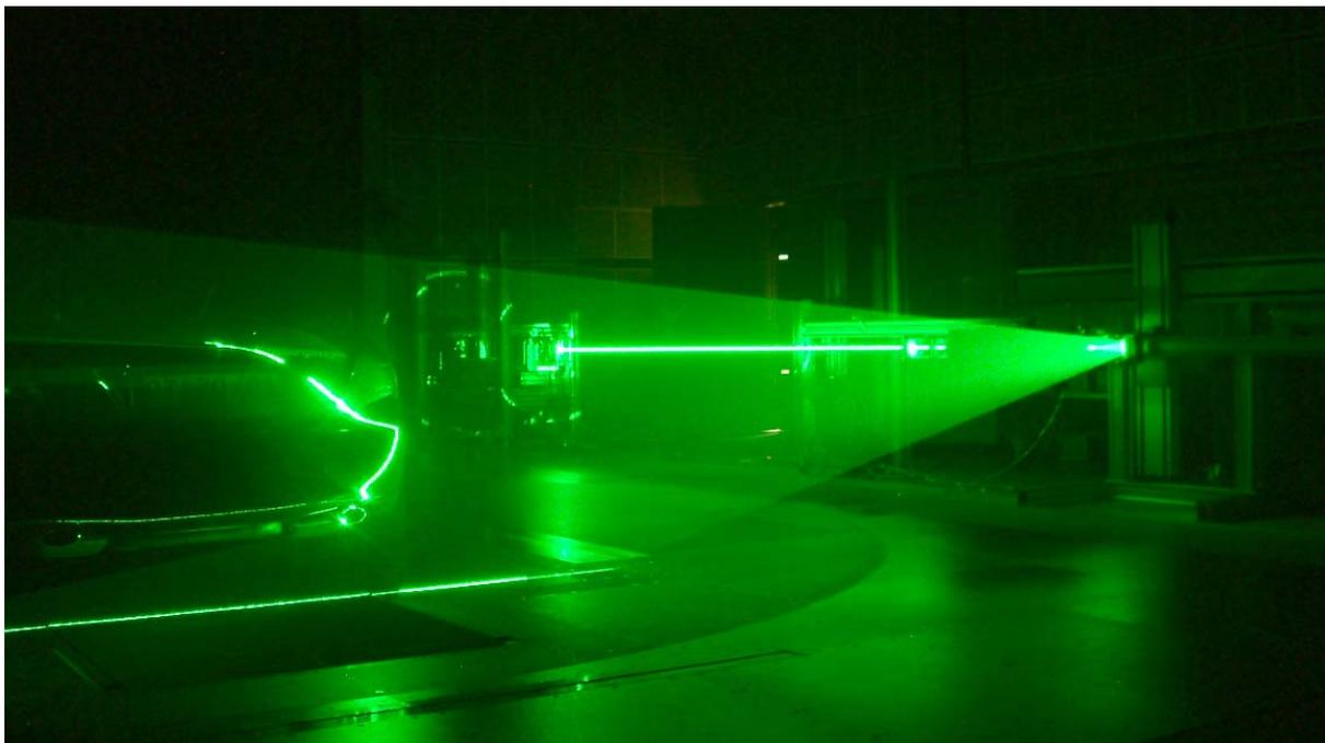
Laser light sheet pulse with high energy for a Stereo PIV measurement during the presentation visible for the participants via video projection inside the control room.
